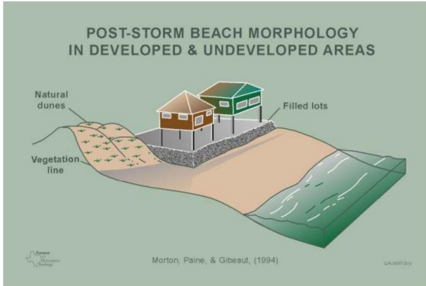
Figure 1.- As the beach retreats, structures prevent foredune formation, which increases the rate of retreat and causes hazardous conditions (from Morton, Paine, and Gibeaut; 1994).
