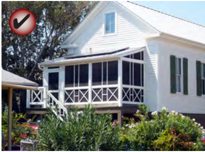
Minimize adverse effects from solar collectors on the character of a historic building.
