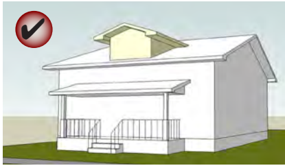
Maintain and repair the original size and shape of dormers.
